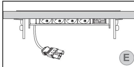
Tight the handles strongly to the surface and verify the Innera Leisure is firmed and cannot be moved.
