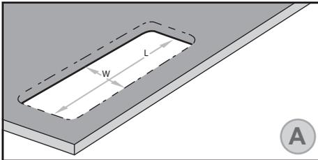
Drill hole into the surface according to the **INSTALLATION TABLE** on page 2. Please verify your purchased item's model No and drill the hole according to the model's cutout dimensions.
