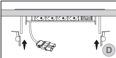
Tight the locking handles by install it on the rails and push it up to the surface.
