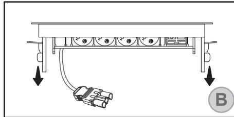
Remove the locking Handles by pulling & Pushing it down the rail before you are Inserting the Innera Leisure into the hole.
