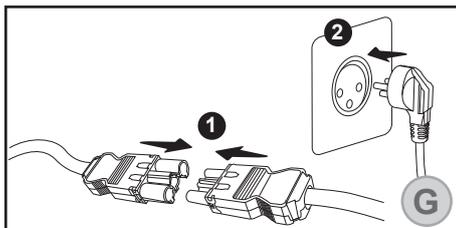
**REMARK:** In case you need to connect the Innera Leisure to a standard socket, you should buy a **starter cable** separately which not included in this Kit and connect it according to illustration above.
