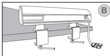
Make sure the locking tripods are tightened strongly to the surface and verify the Exterio Vital is firmed and cannot be rotated.
