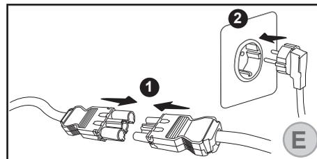
REMARK: In case you need to connect the Exterio Vital to a standard socket, you should buy a **starter cable** separately which not included in this Kit and connect it according to illustration above.
