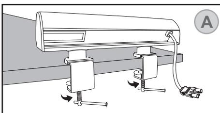
Locate the Exterio Vital on the edge of the desired surface and tight the locking handles of each tripod to the surface by turn them clockwise as in the illustration above.
