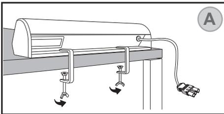
Locate the Exterio Vital on the edge of the desired surface. Assemble each locking hook with nut and screw together and tight them to the surface by turn them clockwise as in the illustration above.
