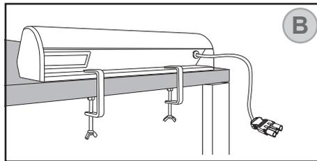
Make sure the locking hooks are tightened strongly to the surface and verify the Exterio Vital is firmed and cannot be rotated.
