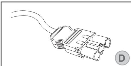
Connect the GST Male connector to power and the Exterio Vital is ready for use.
